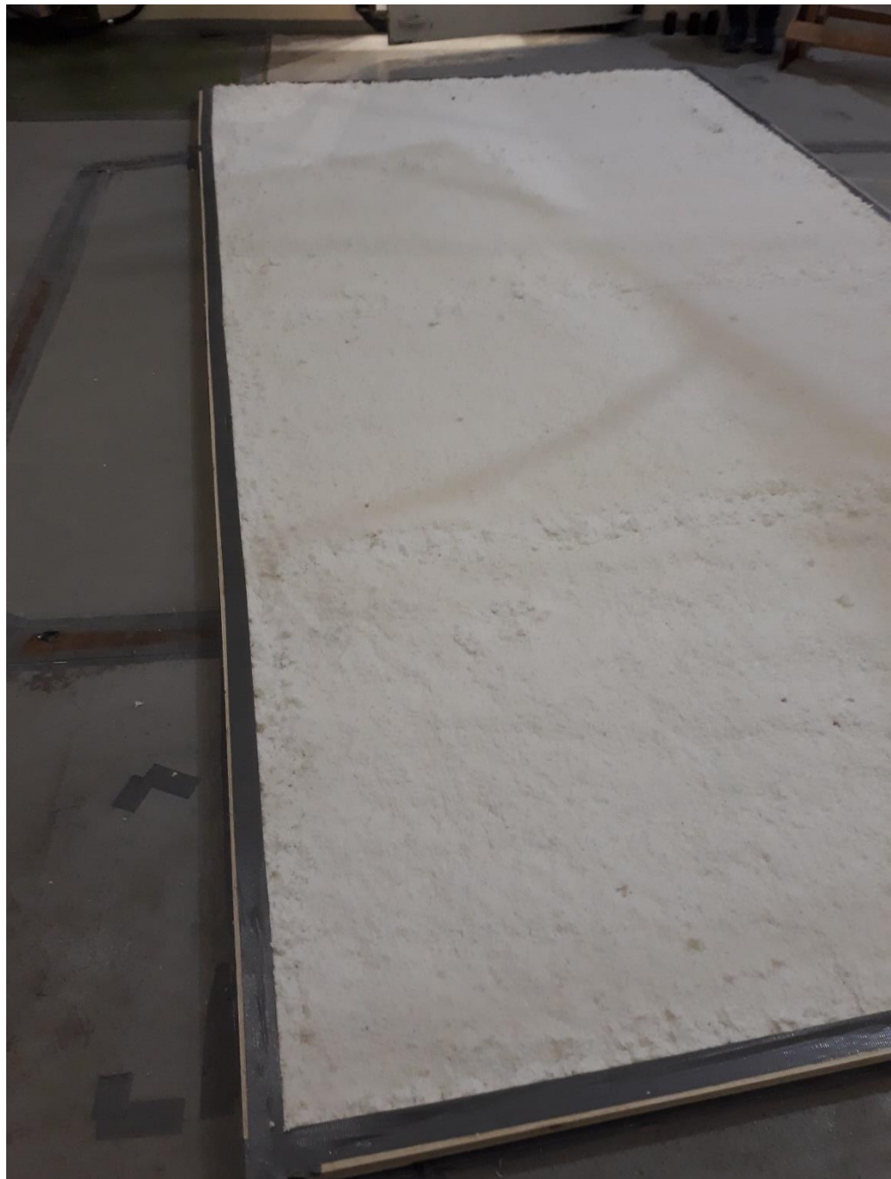
Picture 1. Sample installed to reverberation room.
